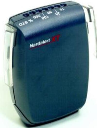
The Nardalert XT RF Personal Monitor operates on the body from 100 kHz to 100 GHz. Its frequency response is shaped to match the FCC MPE limits for Occupational/Controlled exposure.
